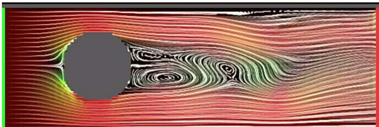
Figure 15: A Vortex-Karman Street. Calculation made for Re = 400 and grid size 119 \times 40 .
