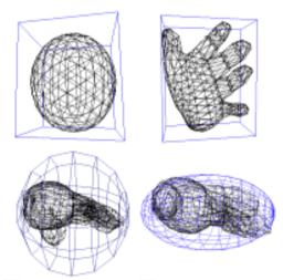
$$V_{el} = \left(\frac{4}{3}\right) \cdot \pi \cdot r_x r_y r_z \tag{4}$$
